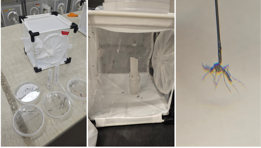
Figure 5: Preparation and mounting of mosquito specimens. The live mosquitoes were provided by the Swedish University of Agricultural Sciences (SLU). Mosquitoes were fed with sugar water instead of blood meal. The right panel illustrates a single freshly killed mosquito mounted on a pin, prepared for hyperspectral scanning.
