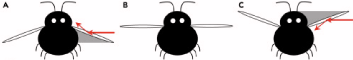
Figure 3.2: Simple visual guide to the wings angle compared to the laser light (red arrows), and when it is blocked as in a) and c), and when no blocking occurs, such as in b). Image from [41].
