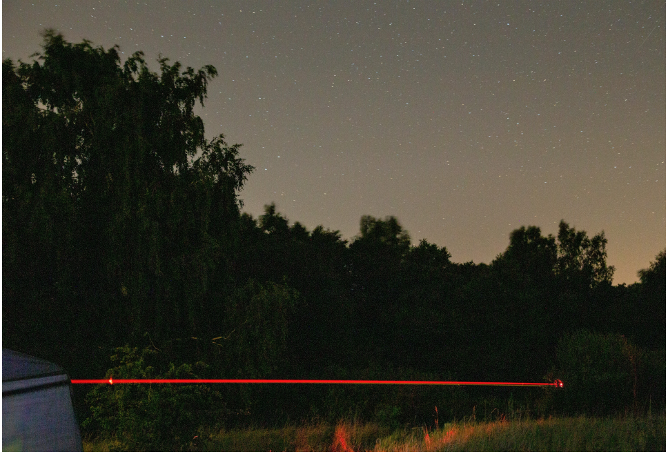
Figure 3.10. The elastic hyperspectral lidar (EHL) at Stensoffa field station, Sweden, measuring wing thicknesses of insects remotely. A flash in the laser beam indicates an illuminated insect. This work is included in Paper III. Image attribution iv .
