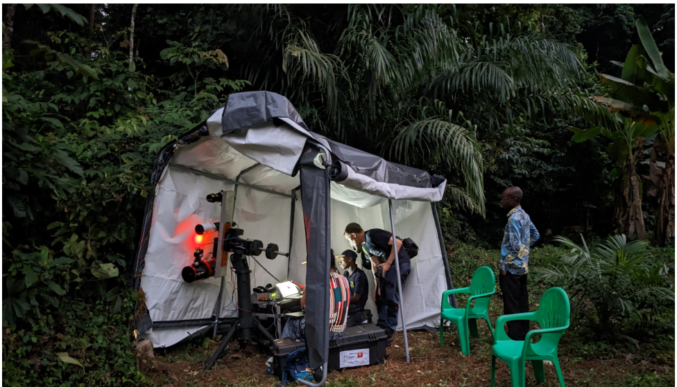
Figure 2.6. Meng, Adolphe, Doria, Mikkel, and Benoit by the lidar, conducting remote sensing of insects in Taï rainforest, Côte d'Ivoire, as part of Paper VI. The motorized tripod was programmed to sweep to different angles, so different heights of the canopy were probed.
